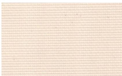
FIBERLUXE™ Architectural Membranes are designed for use as permanent tensioned membranes. These membranes feature a tightly woven fiberglass fabric coated with PTFE - FIBERLUXE™ Membranes allow diffuse natural light in while providing the strength needed for long spans in lightweight construction.
